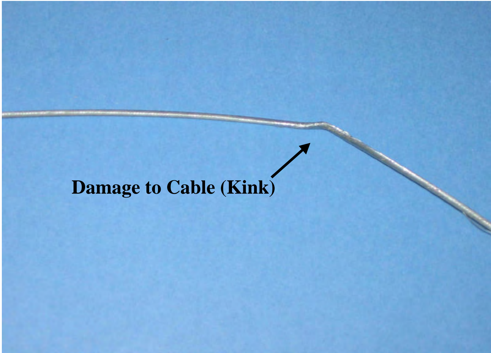
Pic.1 Identification of Cable Damage
