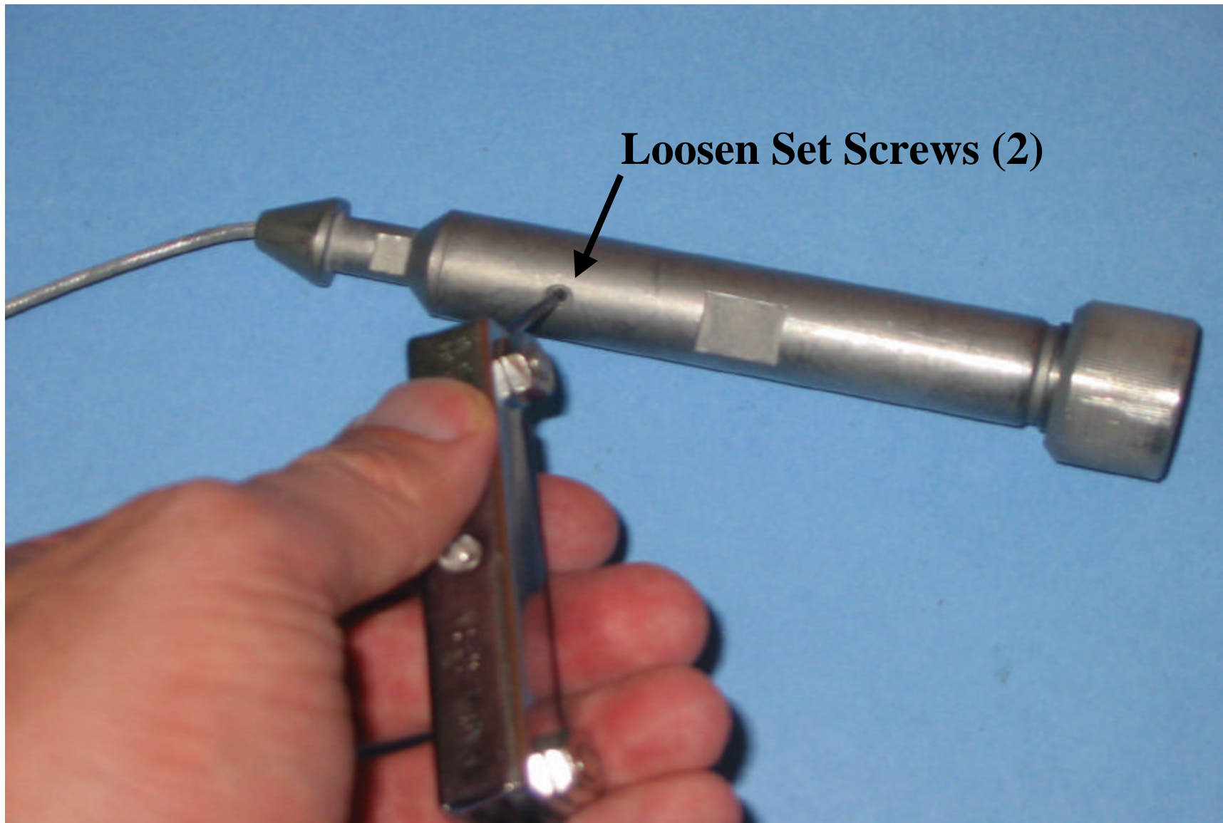
Pic.2 Cablehead Disassembly (1): Loosen set Screws
