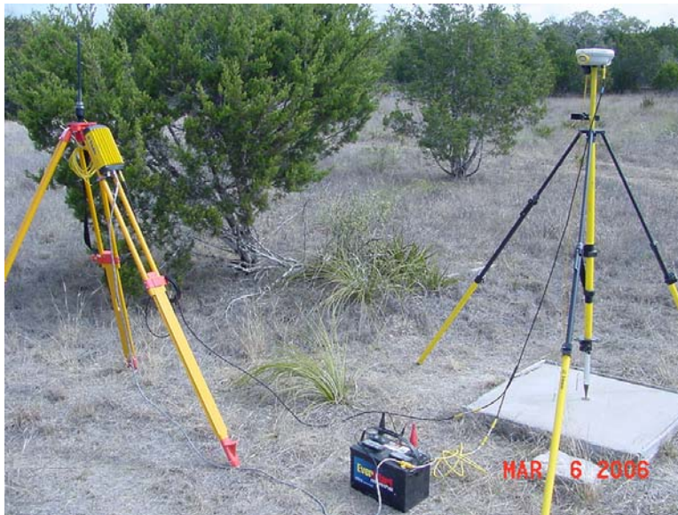
GPS RTK Base Station Setup at CSSA Benchmark 3
