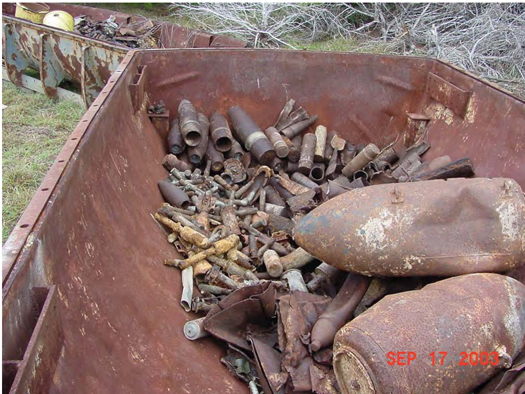
Photo 13-4. Munitions debris items sifted from excavated soil in September 2003.
