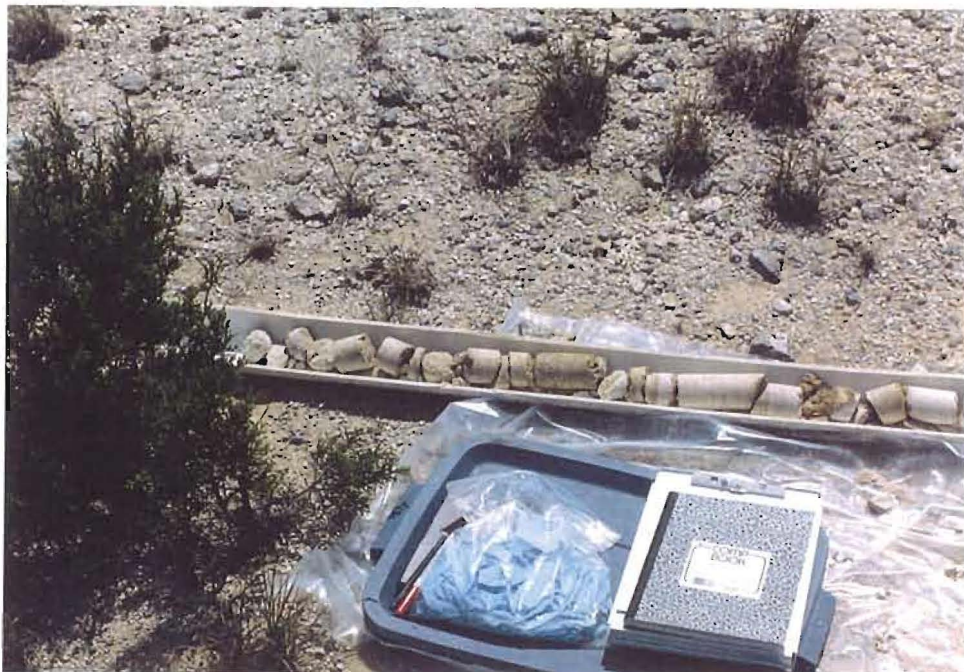
Photo 4. View of core taken from soil boring F14-B1 from 1.5 feet BGL (left side) to 4.5 feet BLG (right side). Light gray cores are limestone and the brownish-yellow layers are marl. Photo taken on 9/9/92 by S. Roberts.
