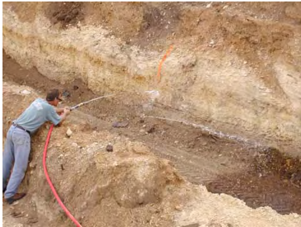
Vegetable Oil applied to Trench 1
