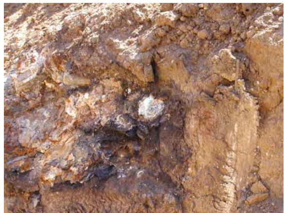
Trench 1 corroded aluminum
