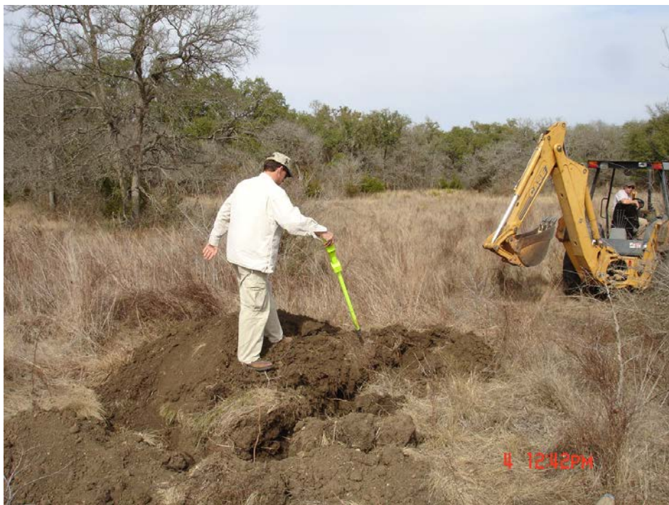
Photo 4. AOC-59 (use of Schonstedt magnetometer in test trench/soil mound area). (January 2006)
